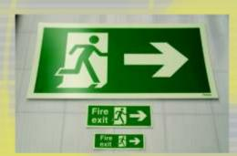
route signs and Norm BS5499-1:2002 for signs other than escape routes. These will indicate the formula to be used. On page 6 of the catalogue, an explanation for this formula and a table with the size of the signs and the relative distances from where they should be visible is presented.
